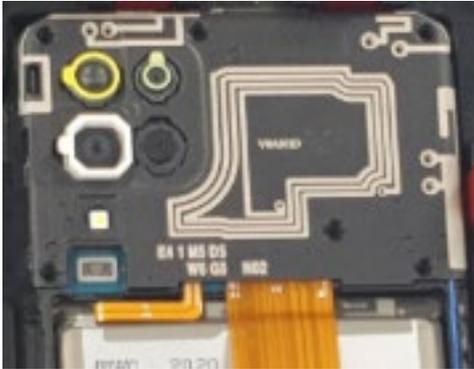
A close-up photograph of the back cover assembly. It shows the camera lens, flash, and various sensors. The assembly is black with white and yellow markings. A yellow flex cable is visible at the bottom.                                                       | <p>Montez le cache arrière haut manuellement.</p>                                                                                                                                                                                    |
